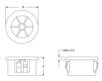
Nylon "ALL-FIT" Adjustable Bushings are designed to protect wire, cable, tubing, or irregular shaped items from sharp, unfinished edges. The specially designed, resilient multiple supports absorb shock and vibration and adjust to accept various diameters and shapes. The All-Fit Bushing is equipped with multiple locks to positively snap in panel thicknesses ranging from 1/32" to 1/8". Molded in heat stabilized nylon UL94V2 black.
